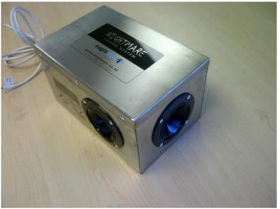
The sound system for the control of roosting pigeons:
